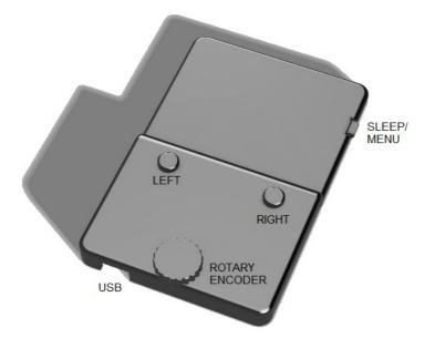
MAKE SURE TO CHARGE YOUR LEDBOY FULLY BEFORE PROCEEDING, WHEN FULLY CHARGED, THE CHARGE LED ON TOP THE USB PORT TURNS OFF, IF THE LED IS ON, THE BATTERY IS CHARGING.
